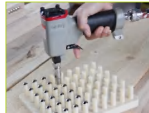
Step2 Put the nose on the studs
