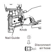
③Open the nail guide and remove dust. Lubricate the nose opening and feeder shaft.
