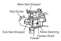
①Lubricate the feeding surfaces of the nose and the nail guide after cleaning.
