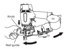
(2) Adjust the position of the nail holder according to the nail length.
