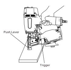
(2) Adjust the air pressure to 70 psi (4.9 bar 5 kgf/cm²). Connect the air hose.
