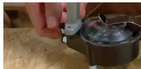
Step2 Adjust air inlet
