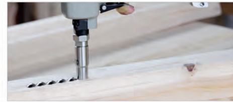
Step3 Actuate the trigger to shoot
